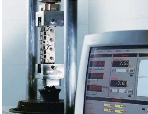
Figure 1: The high-frequency pulsometer determines the fatigue strength
